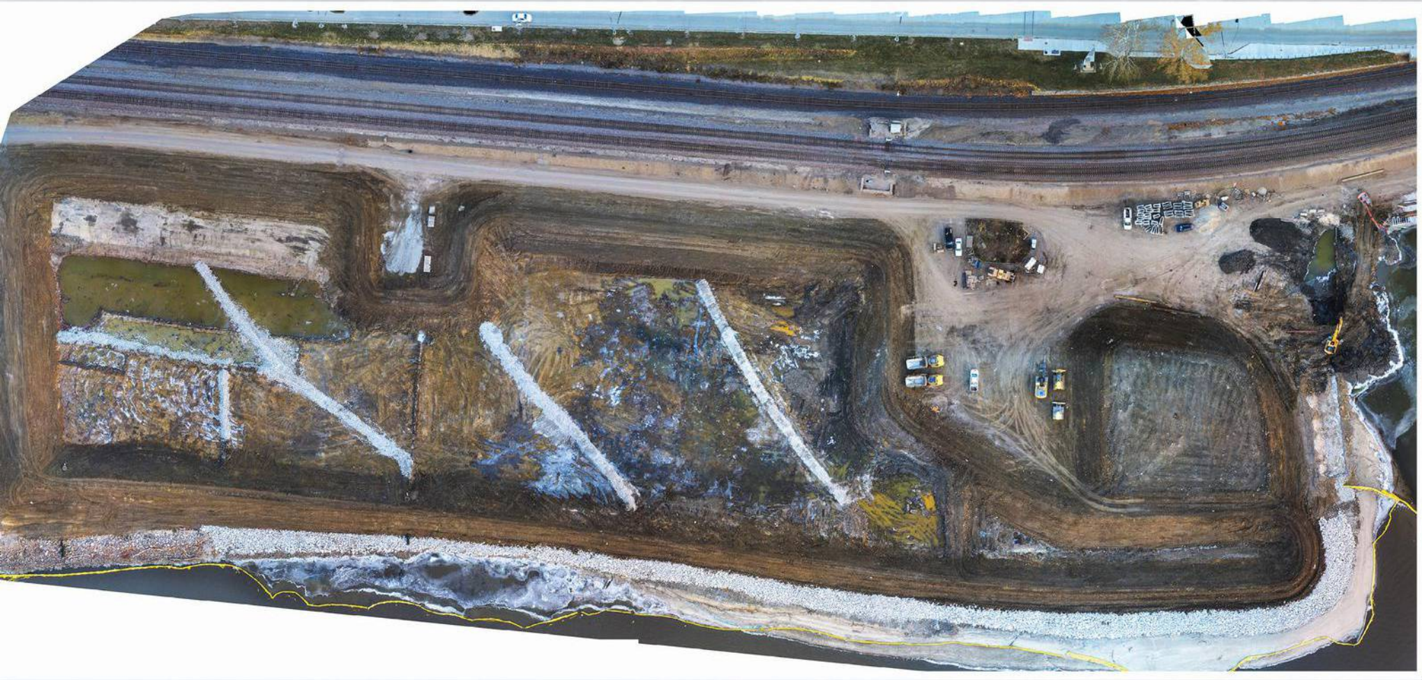
The on-site dredge basin in December 2021 before dredging began, showcasing the exposed rock weirs
